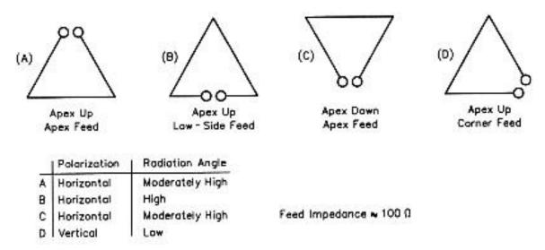
Mine is installed according to figure A, giving me horizontal polarization and a "Moderately high" radiation angle. This is the lowest radiation angle that can be achieved with an apex up Delta Loop using horizontal polarization.
